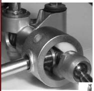
5. Remove/tighten the knuckle supporting the handle.
